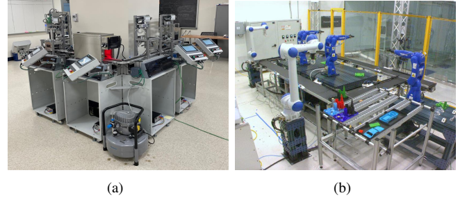
Fig. 1. Testbeds to be modernized with hardware acceleration. (a) Cyber-Physical Lab (CPLab) for assembling cellular phones, consisting of eight cells. Cells 1-4 are shown in the figure, each containing a Human-Machine Interface (HMI), a camera, and a PLC. Workpieces are conveyed between cells, orchestrated by a Manufacturing Execution System. (b) The Future Factories Lab (FFLab) is a testbed with five robotic arms for autonomous rocket assembly and disassembly, showcasing multi-robot coordination and conveyor-driven part handling in a closed-loop manufacturing system.
